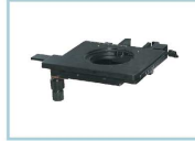
CFM261201 MANUAL STAGE Manual Stage, dimensions: 180×150mm, XY 90×60mm travel, the clamp opening is from 25mm(10") to 37.2mm(15.1").
